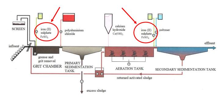
Struvite (MAP or magnesium-ammonium-phosphate) recovery only possible in municipal wastewater treatment plants with enhanced biological phosphorus removal (EBPR). (Wilfert et al., 2018)
