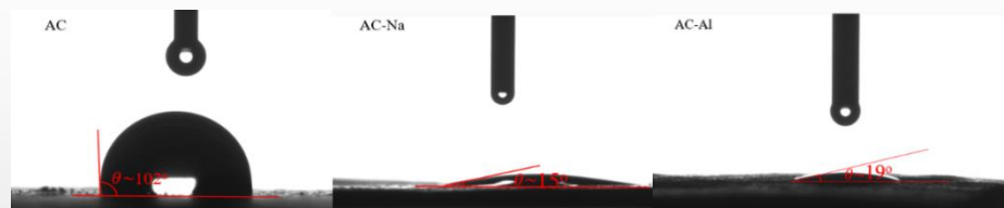
Contact angle of a water droplet on the surface of the AC pristine electrode and electrodes after surface modifications.
